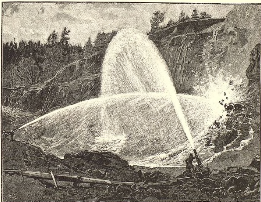
HYDRAULIC MINING IN THE MOUNTAINS OF CALIFORNIA.
