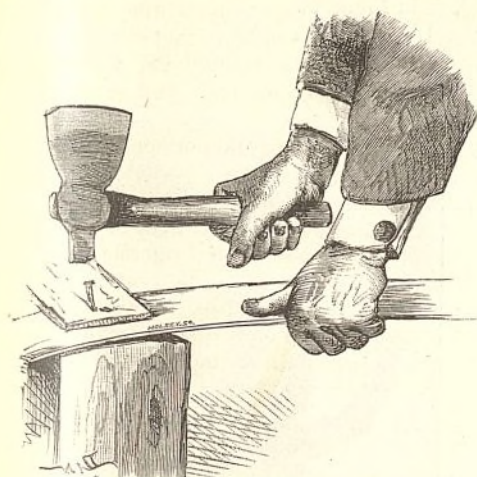
FIG. 1. HOW TO NAIL THE CROSS-PIECES ON.
