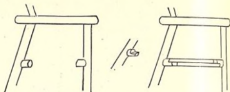
DIAGRAM SHOWING PHAETON'S METHOD OF REPLACING THE CHAIR-ROUNDS.
