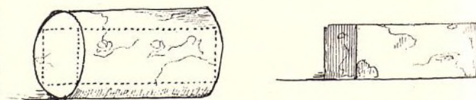
DIAGRAM SHOWING HOW A MINIATURE BRICK MAY BE CUT FROM A CORK.
