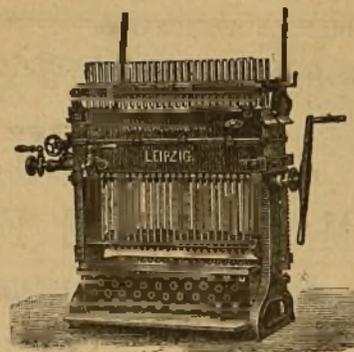
MÁQUINAS PARA FABRICAR BUJÍAS
