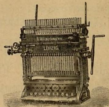
MÁQUINAS PARA FABRICAR BUJÍAS
