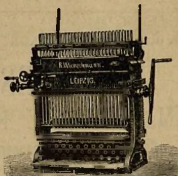
MÁQUINAS PARA FABRICAR BUJÍAS
