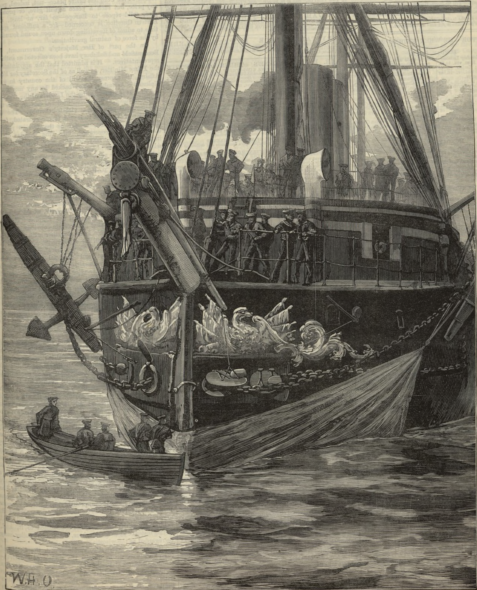
THE COLLISION OFF FOLKESTONE BETWEEN TWO GERMAN IRONCLADS: THE KÖNIG WILHELM, SHOWING THE DAMAGE TO HER BOWS.
